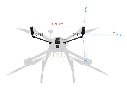
Set the position of the main and secondary antennas for the SIYI RTK Positioning and Orientation Module:
