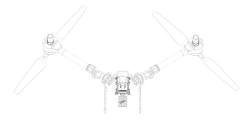
Refer to the image above to securely mount the RTK mobile end on the aircraft body, ensuring it does not wobble. The arrow on the RTK module should align with the installation direction of the
