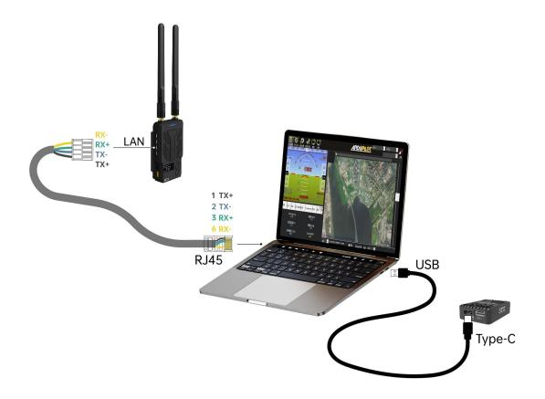
Refer to the above diagram to set up the F9P RTK base station. The base station communicates with the PC ground station and transmits the real-time position of the RTK base station to the flight controller via the data link.
